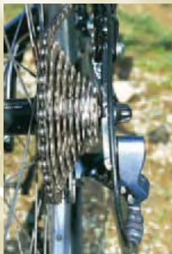
Large sprocket The chain is moved to the largest sprocket by the pull of the cable.
