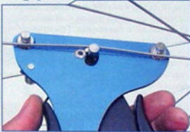
Park Tool TM-1 Tension Meter flexing spoke to determine tension
