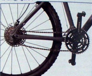
By-pass derailleur to create a make-shift one speed
