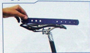
Use straight edge to extend saddle line
