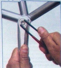
Check security of one-key release system crank arm cap
