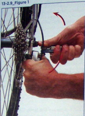
Bend hanger back until visually straight
