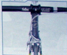
Housing enters stop in a straight line, indicating a good length
