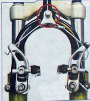
Straddle wire carrier for cantilever calipers
