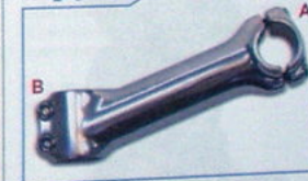
Common threadless stem. (A) Handlebar binder bolts, (B) Stem binder bolts
