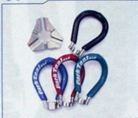
Spoke wrenches for various sized spoke nipples
