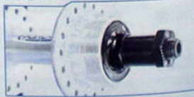
Rear hub threaded for freewheel
