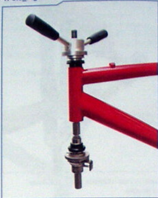
Arrangement of cups and pressing guides for the HHP-2
