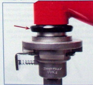
This cup is not fully seated into frame
