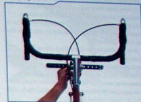
Straight edge is parallel to bar, which makes stem aligned
