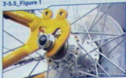
Solid or non-quick release axle on derailleur type bike
