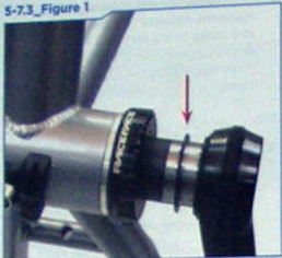
Moveable chainline spacer installed next to left crank
