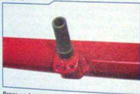
Braze on for brake mounting
