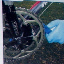
Scrub chainrings with solvent on the brush
