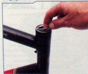
Removing the integrated headset bearing
