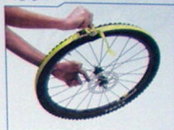
Use a strap to apply even pressure on tubeless tires that are difficult to inflate
