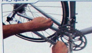
Use the frame to control bending of the hanger
