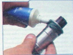
Greasing the threads of the bottom bracket
