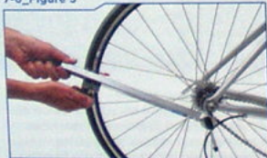
Set DAG-1 to reference rim at the nine o'clock position
