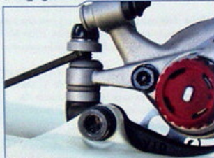
Ball and socket system for pad and caliper alignment to rotor
