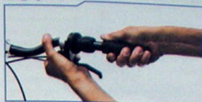
Wet grips with fluid and quickly push into place
