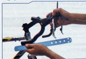
Adjust lever height for comfort
