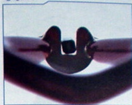
If spoke wrench is large for the nipple, damage may occur
