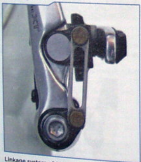
Linkage system of Shimano® V-brake system
