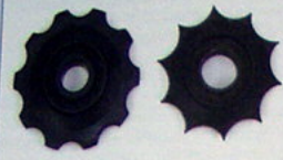
Unworn pulley wheel on left and extremely worn pulley on right
