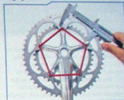
Measure pentagon cord by measuring bolt-to-bolt
