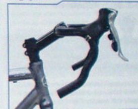
Upper limit of drop bar rotation
