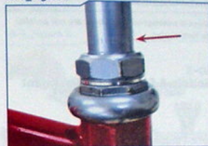
Stem is too high, "max height" must not be visible
