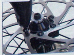
Secure bolts using Torx driver
