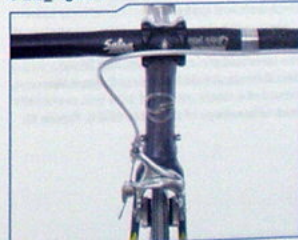
Housing passes housing stop, indicating housing is too long
