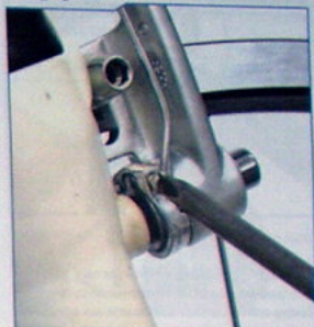
Use screw to change spring tension when centering pads to rim
