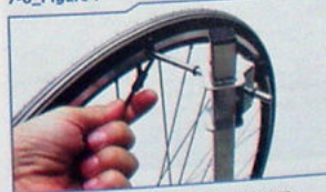
Use a 4mm gauge to check the tolerance
