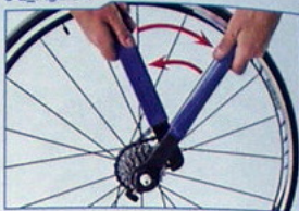
Loosen locking while holding cassette sprockets
