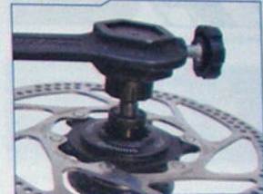
Shimano XTR locking system for rotor mounting
