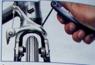
Center pads to rim with setscrew in brake bridge
