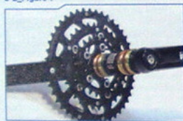
Three-piece crankset, consisting of two arms and one spindle
