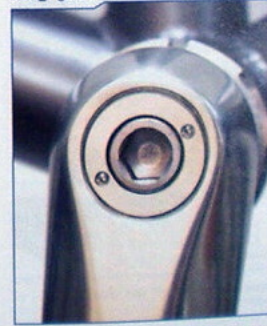
One-key release system with crank arm cap and crank bolt
