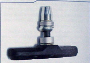
Ball and socket system of threaded brake pad
