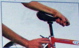
Test saddle rotation with only one hand, not two
