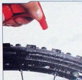
Use soapy water to help bead seat into rim
