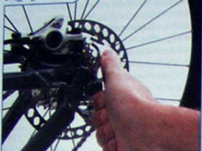
Re-bending a warped rotor
