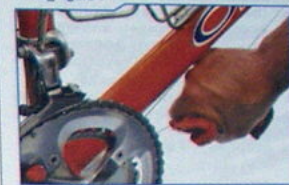
Pull derailleur cable by hand to isolate limit screw performance
