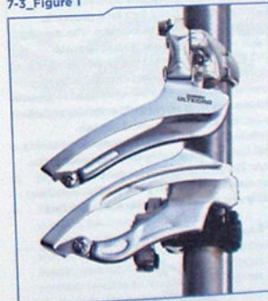
The shallow cage derailleur cage on top and the deep cage below
