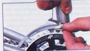
Set height for 1-2 millimeters at the closest point
