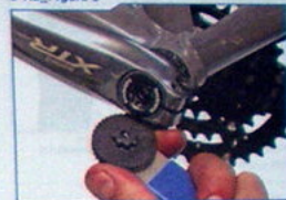
BBT-9 tool is used to remove crank cap
