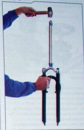
Pressing the fork crown race
