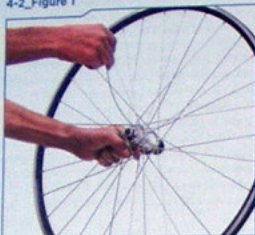
Bend spoke to lace into wheel
