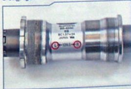
Bottom bracket marking indicating side of bike
