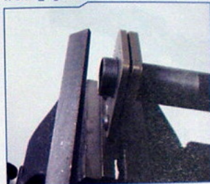
Bevel end of fork thread
