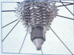
Use skewer to hold tool firmly in place
