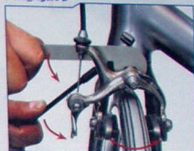
Centering sidepull with centering flats on brake stud
