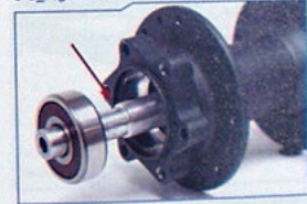
Non-threaded axle with a cartridge bearing
