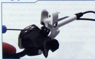
Reach screw adjustment on the Shimano® brake lever
