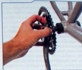
Install crank with spindle through both bearings
