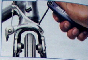
Center pads to rim with setscrew in brake bridge
