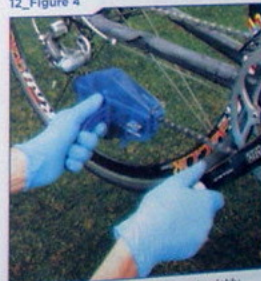
Chain cleaners can thoroughly and quickly clean the chain
