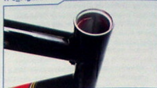
Head tube of an integrated headset bike
