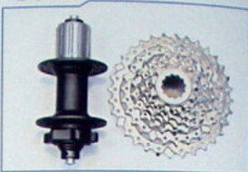
Freehub body and hub with cassette sprockets
