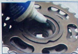
Freewheel internal threading. Grease threads before installing
