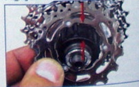
Align wide spline inside sprocket with wide space on freehub body
