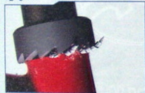
Facing the head tube for better bearing alignment
