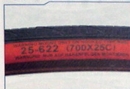
ISO (ETRTO) sizing on tire label along with French sizing system
