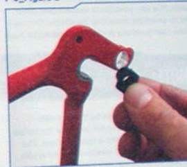
T-nut thread repair of a stripped hanger
