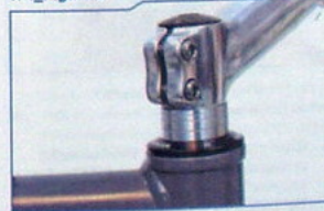
Bike with low-profile threadless headset
