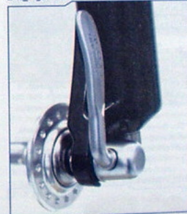
Skewer must be oriented to allow lever to fully close, even with wide fork ends
