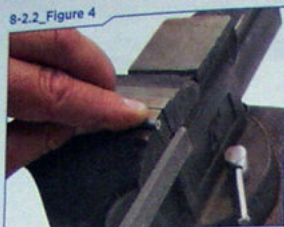
File brake coil smooth to eliminate burr from cutting
