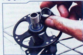
Threaded sleeve nut holding axle to cartridge bearing
