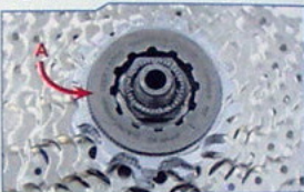
Locking holds cassette sprockets secure to freehub body. (A) Locking
