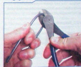
Flexing wound-type housing opens coils for the cutters
