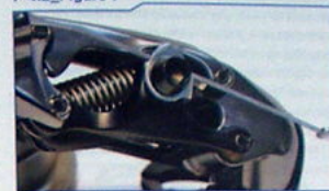
Derailleur cable flattened by pinch mechanism of plate and bolt
