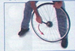
Turn tool counter-clockwise to remove freewheel from hub
