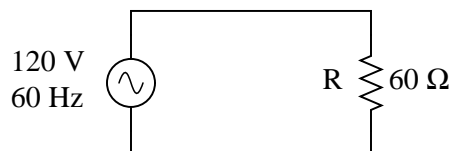
Figure 11.1: Ac source drives a purely resistive load.
