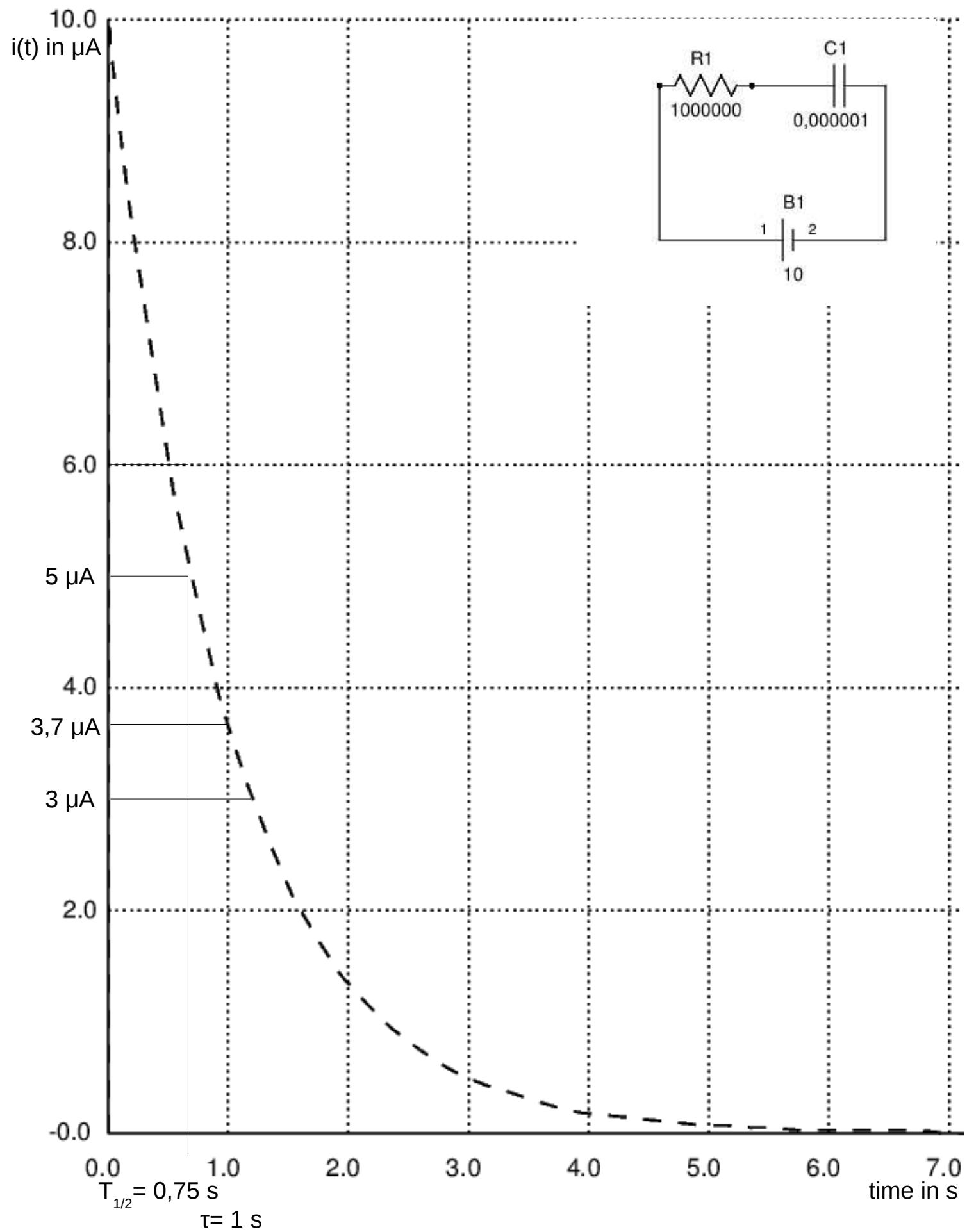
Calculation of  $i(t)$  assuming a half-life period graphically determined of  $T_{1/2} = 0,75$  s
