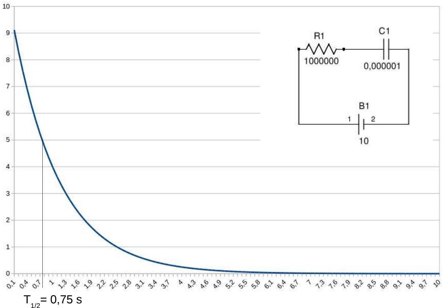
The derivative of the function must be negative, since it's falling.
