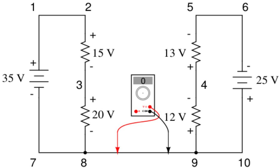
*Measuring voltage from point 8 to point 9 (0 volts)*
