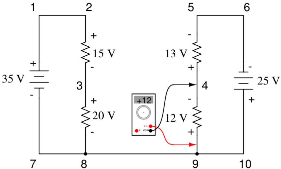
*Measuring voltage from point 9 to point 4 (+12 volts)*
