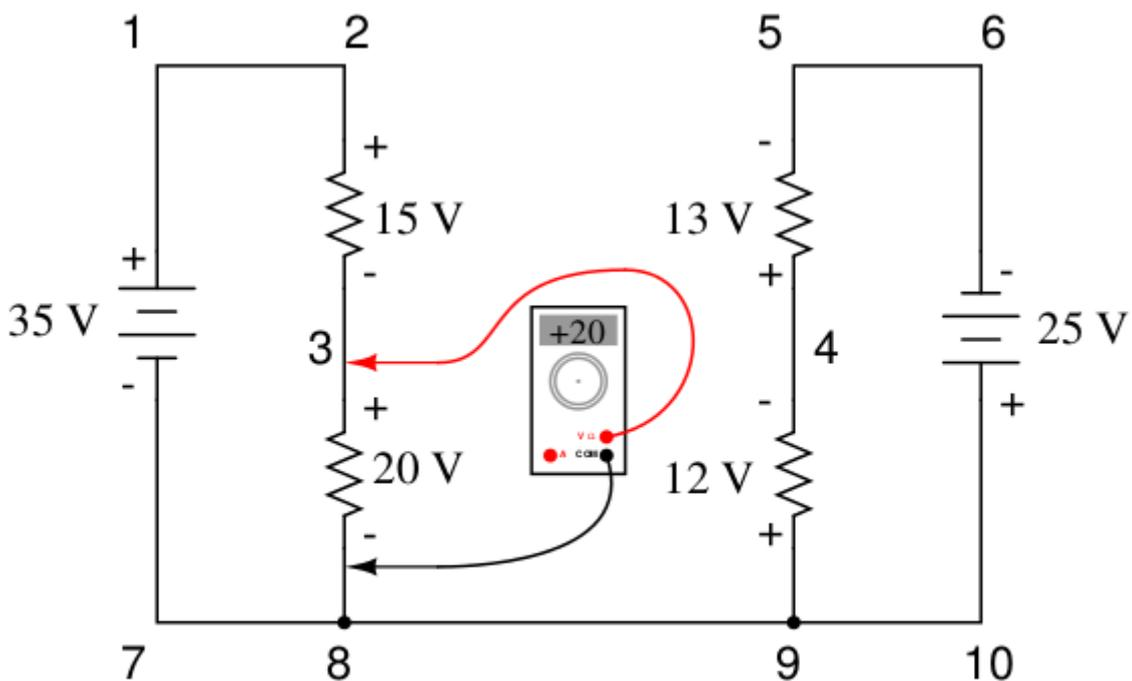
*Measuring voltage from point 3 to point 8 (+20 volts)*
