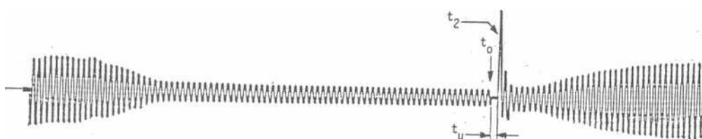
Figure 4a Star-Delta Start - Open Transition
